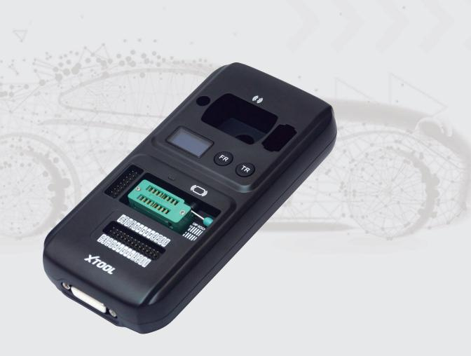
Powerful in functions and fashionable in appearance, KC501 is a professional Key & chip programmer which can not only read,write keys and read key remote frequency, but also generate dealer keys. It support read and write MCU/EEPROM chips, read and write Mercedes Infrared keys. Moreover, it support PC connection which brings you better user experience.
