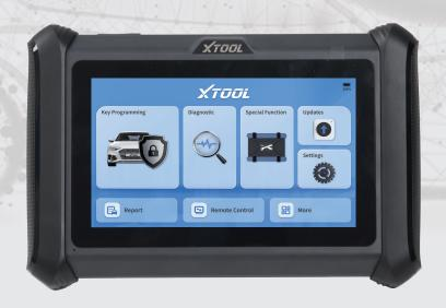
X100PADS is an automotive key programming device with a 7-inch LCD display and Android 10 OS, which is designed for locksmiths, vehicle owners and car mechanics. It supports vehicle programming for 2,000+ models under 60+ car manufacturers, providing solutions on reading immobilizer data, extracting pincode, add keys, all keys lost, remote programming, etc.
