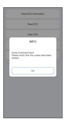
The trouble codes cannot be cleared without eliminating all the troubles, the diagnostic tool can always read those codes as those codes are saved in ECU.
