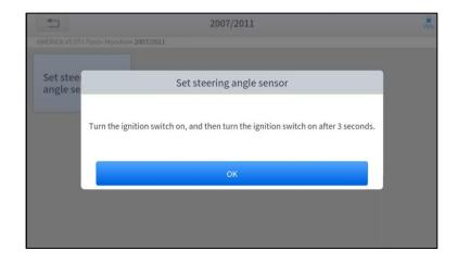
1. Message of 'Function execution is completed' displayed when SAS reset function has successfully completed.
