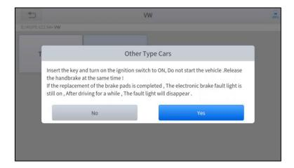
Enter the Enter maintenance mode menu and release the handbrake brake. And press OK after completing the instructions shown.
