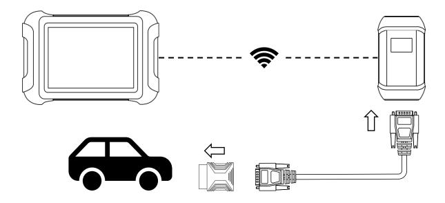
The scan tool must be connected to the vehicle's OBD-II port so that the tablet can establish correct vehicle communication. Please perform the following steps:
