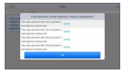
Enter the Change the value of cylinder menu of the replaced injector(s), enter the new 5-digit value, and then press OK.
