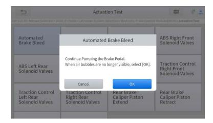
Continue pumping the brake pedal, when air bubbles are no longer visible, select OK to enter next bleed procedure for left front wheel
