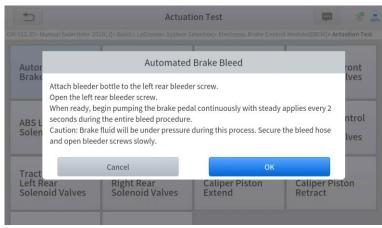
4. When ready, click "*OK*" to enter the bleed procedure, and pumping the brake pedal continuously with steady applies every 2 seconds during the entire procedure
