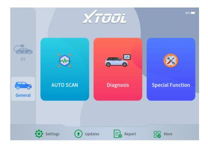
The diagnostic application can read ECU information, read and clear DTC (Diagnostic Trouble Codes) and check live data and freeze frame data. The Diagnostic application can access the ECU of various vehicle control systems, including the Engine, Transmission, Anti-lock Braking System (ABS), Airbag Safety Restraing System (SRS), Electronic Parking Brake system (EPB) and perform many types of actuation tests.
