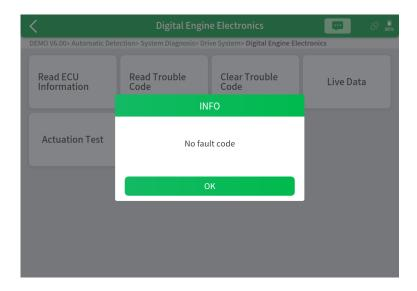
In the process of diagnosis, if the device shows "System is OK" or "No Trouble Code", it means there is no related trouble code stored in ECU or some troubles are not under the control of ECU. Most troubles are mechanical system troubles or executive circuit troubles. It is also possible that the signal of a sensor may be inaccurate but within limits, which can be examined using Live Data.
