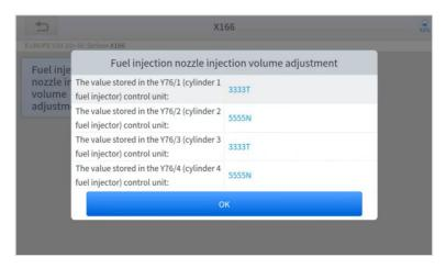
Figure 5-25 Sample of injector coding function (screen 4)
