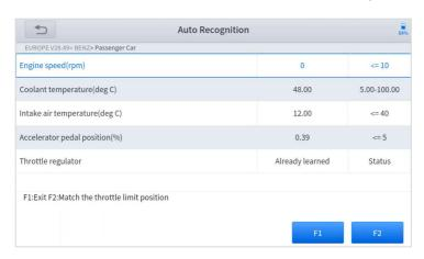
Figure 5-21 Sample of throttle function (screen 2)
