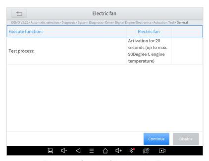
Figure 4-15 Sample of the Actuation Test
