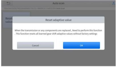
Figure 5-26 Sample of gearbox matching function (screen 1)
