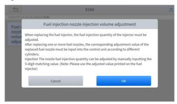
Figure 5-22 Sample of injector coding function (screen 1)
