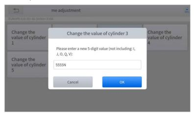
Figure 5-24 Sample of injector coding function (screen 3)
