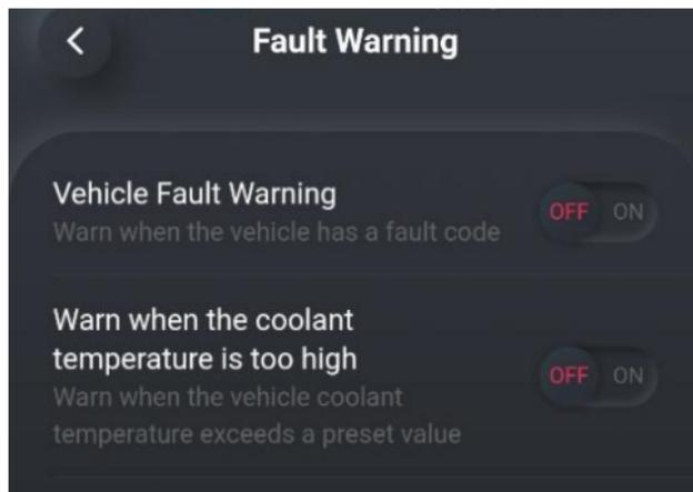
▼ AD10 supports alarm prompts when a fault code or abnormal coolant temperature occurs. You could choose to turn it on or off.
