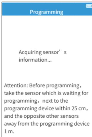
Via direction key select the waited programming tire pressure sensor, press OK key to continue.
